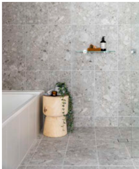
Image 7. Bathroom with slip resistant, hobless shower recess in the corner of the room with a shower screen that can readily be removed at a later date (Courtesy of Stockland Communities)
