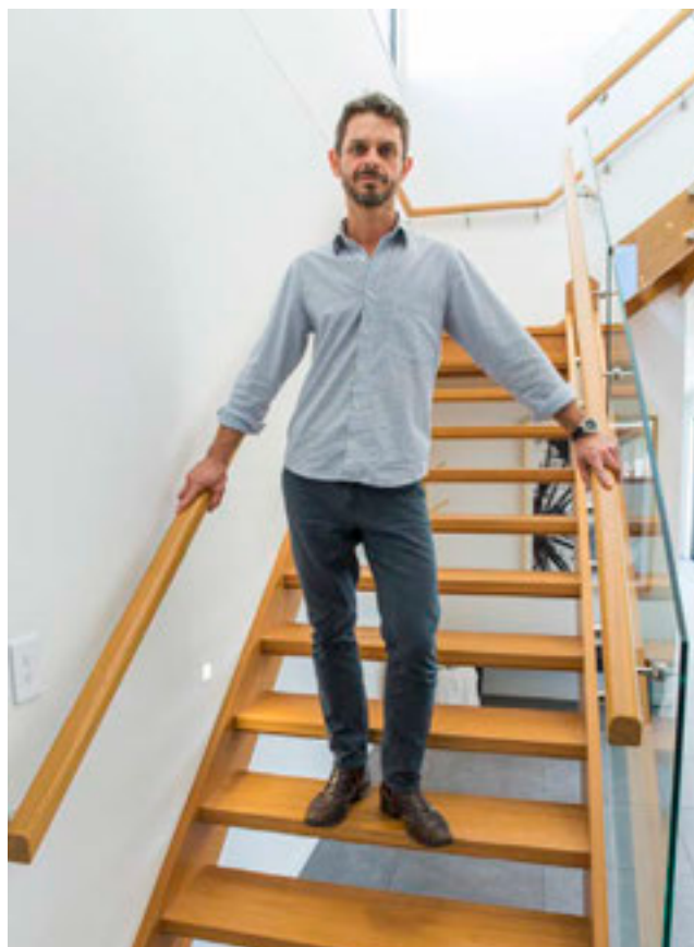
Image 9. Internal stairway designed to reduce the likelihood of injury with adjoining a load bearing wall to enable future adaption (Courtesy of Parent to Parent Assoc. QLD - P2P Housing Team)
